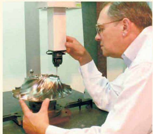
A digital coordinate measuring machine is used to inspect impellers.
