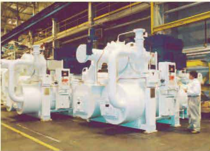
Two of three 8,500 CFM (14,400 m 3 /hr) air compressors that supply compressed air for snowmaking, ensuring a plentiful amount of quality snow for the 2002 Winter Olympics.
