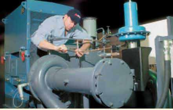
Easily accessible bolting facilitates the removal of the gear case cover.
