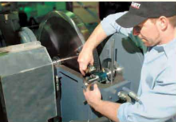
The bearing top half can be taken off after removing two screws. The bottom half of the bearing can be rolled out and removed from the casing for inspection. The two-piece seal assembly can be removed by sliding it into the bearing cavity area; then follow the same procedure that was utilized for removing the bearing.
