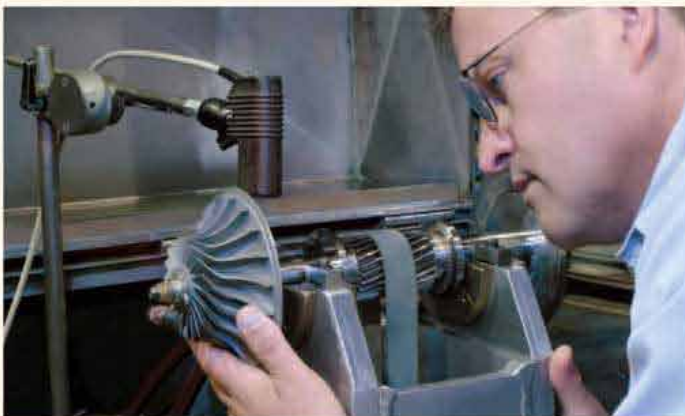
Rotor assemblies are dynamically balanced.
